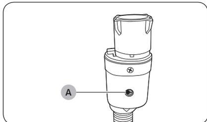
The aqua hose alerts users of a risk of water leaks. It senses the water flow and turns red on the centre **indicator (A)** in case of a leak.
