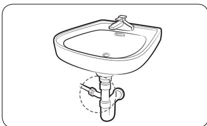
2. Connect the hose adapter directly to the drain pipe of the wash basin.
