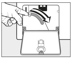
■ Push the emergency drain lever downwards and hold until no more water runs out.
