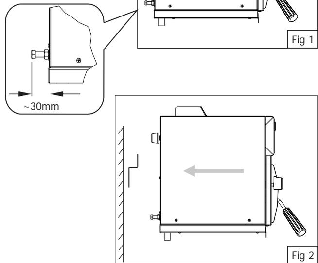
4. Lift Salamander onto wall bracket, lining up black plastic spacers on salamander with mounting notches in bracket.
