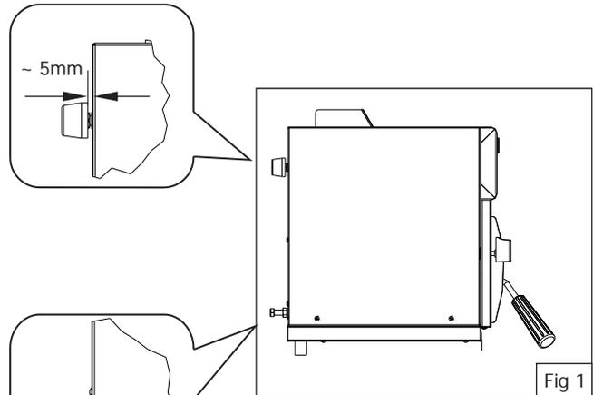
3. Fit two adjusting screws / bolts into nutserts at bottom rear corners of unit. These should protrude approximately 30mm from rear of Salamander.
