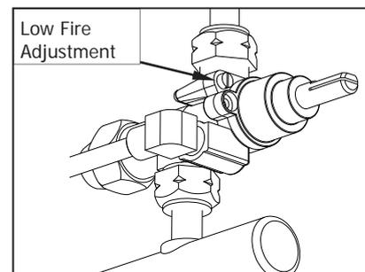
**NOTE: 'Low Fire Screw' should be sealed with coloured paint on completion of low fire adjustment.**
