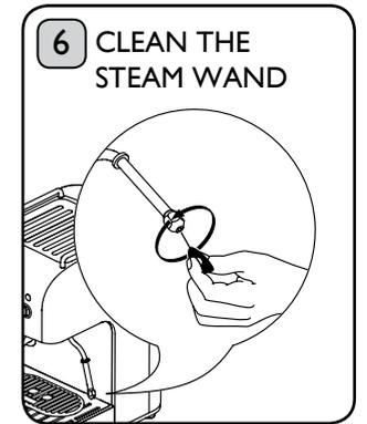
Use the steam pin to remove dried milk from inside the steam wand. Use the measuring spoon to place the nut back on the steam wand. Screw clockwise until tight.
