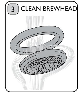
Thoroughly clean the showerhead and gasket to remove any coffee grounds. Use the filter pin to unblock or rinse in suds.
