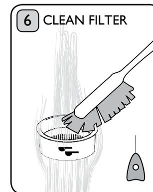
When using the filter holder, knock out the grounds over a bin. Rinse the filter under running water to remove any coffee grounds. Use the filter pin to unblock if required.
