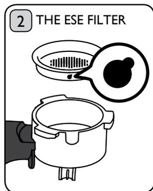
Select the ESE pod filter and snap into the filter holder.
