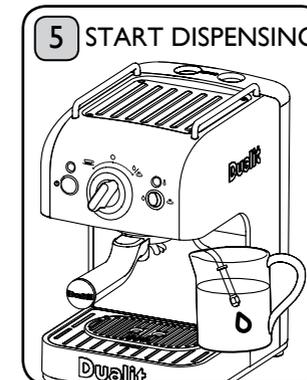
Turn the control knob to the steam/water position to start the water flowing. You will hear the pump; this is quite normal.
