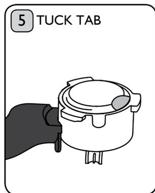
Make sure all the paper is tucked inside the filter before attaching the filter holder to the brewhead.
