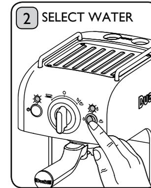
Set the steam/water selector switch to the water setting.
