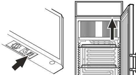
The light can be switched on and off by pressing the switch.
