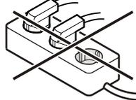
Do not use stand-alone inverters (conversion of direct current to alternating current/three-phase current) or energy-saving plugs. Risk of damage to the electronic control system!
