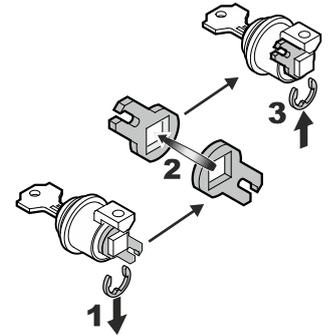
**12.** Remove door latch, turn over and re-assemble.
