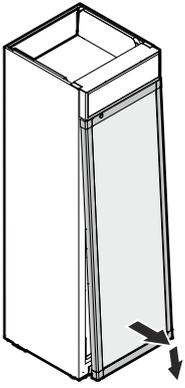
**3.** Move the bottom of the door forwards and remove it downwards.
