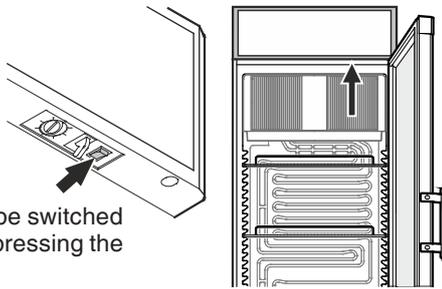
The light can be switched on and off by pressing the switch.
