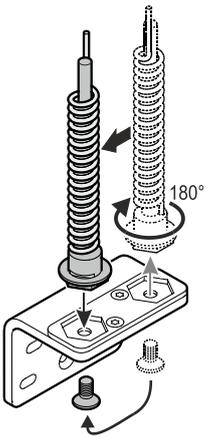
**6.** Unscrew the hinge pin, turn it through 180° horizontally and insert into the left-hand opening.
