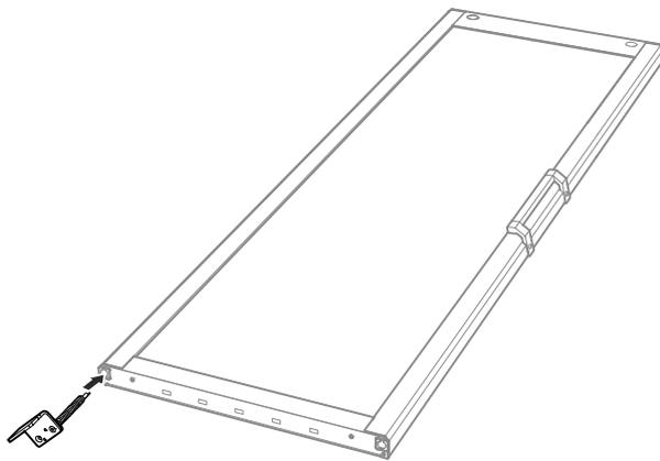
**19.** Insert the hinge bracket as shown in the illustration and hold it.
