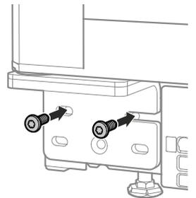
**Adjusting the lateral tilt of the door**
