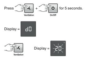
The refrigeration unit switches on. The temperature display flashes.
