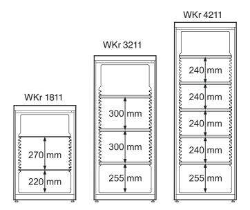
The storage capacity stated is only possible with the grid shelves in this configuration.
