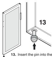
13. Insert the pin into the left-hand door mounting. Use your index finger to hold the pin while you are assembling the door.
