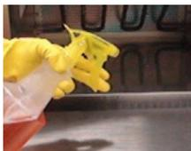
3. **Wear rubber gloves and safety glasses.** Spray oven door and cavity with ACP Oven Cleaner (CL10). Avoid spraying into perforations. Allow cleaner to soak for 2 minutes.
