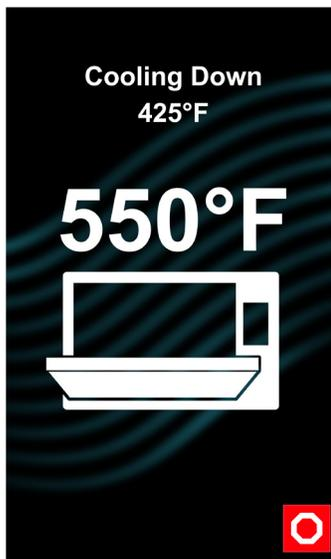
"Cooling Down" screen appears and stays on until oven temperature is below 200°F (95°C)
