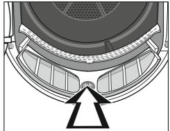
Push the lower fluff filter in completely and lock it with the yellow dial.
