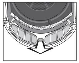
Pull the fluff filter forwards to remove it.
