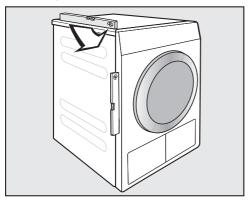
The appliance must stand perfectly level on all four feet to ensure safe and proper operation.
