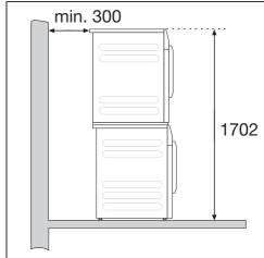
A stacking kit\* is required. This must be fitted by a Miele authorised technician.
