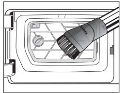
Carefully vacuum up any visible fluff or soiling. Use a dusting brush or the narrow crevice nozzle.
