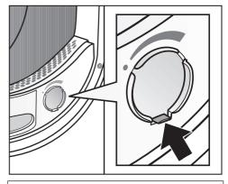
If you are not using a fragrance flacon: push the tab down completely (see arrow) so that the socket is closed. Otherwise, fluff will accumulate here.
