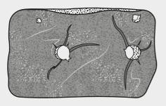
Fluff will blow into the heat exchanger through cracks and tears and will cause obstruction.
