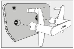
■ Pull the handle out of the fluff filter.
