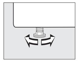
The screw feet can be adjusted to compensate for unevenness in the floor.
