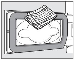
Use a damp cloth to remove any fluff. Make sure that you do not damage the rubber seal when doing this.
