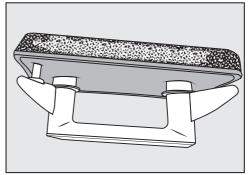
Residues arise from laundry fibres and traces of detergent components which can clog the filter. They can be found on the front and side edges of the filter. In extreme cases, they can form stubborn crust.
