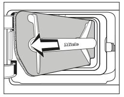
2 Pull the fluff filter out at an angle.
