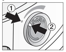
■ Turn the outer ring anti-clockwise until the markers ① and ② line up.
