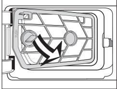
Use the handle to pull out the filter insert <u>at an angle</u> forwards and to the right.
