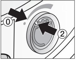
■ Turn the outer ring anti-clockwise until the marker ② is in position ③.
