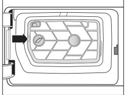
3 Press the frame of the filter insert in at the positions marked PUSH until it audibly engages.
