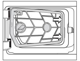
1 Use the handle to slide the filter insert to the right at an angle behind the edge.
