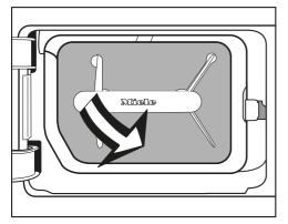
① Use the handle to pull out the fluff filter at an angle forwards and to the right.
