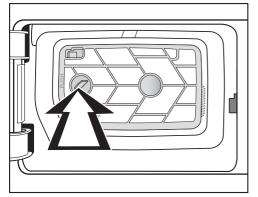
2 Then press on the handle until the filter is secured in position on the left.
