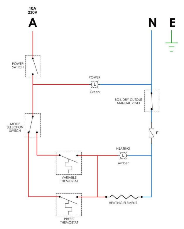
NOTE: This circuit diagram has been provided for reference and to assist qualified service and repair agents only. Under no circumstances should person's not suitably qualified attempt repairs to any electrical equipment.
