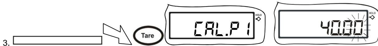
4. Enter in calibration weight from 25% to 100% full capacity.
