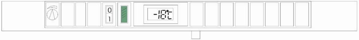
The thermostat can be positioned from app. -15 to -25°C.
