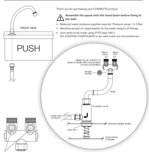
After installation turn the adjustment screws until the desired water temperature delivery to the spout is achieved.
