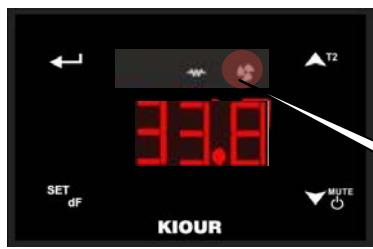
The heated cupboard fan is on.
